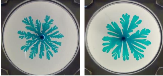
図1 9.7wt% HEC(高粘性流体)と水(低粘性流体)のVF実験 Fig.1 VF experiment of 9.7 wt% HEC (more viscous) and water (less viscous)
